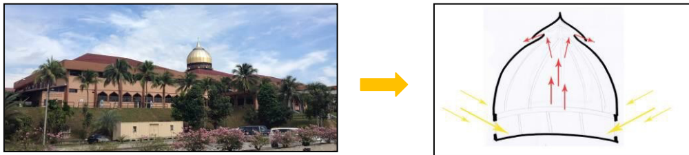
Fig .2. Dome for stack effect
