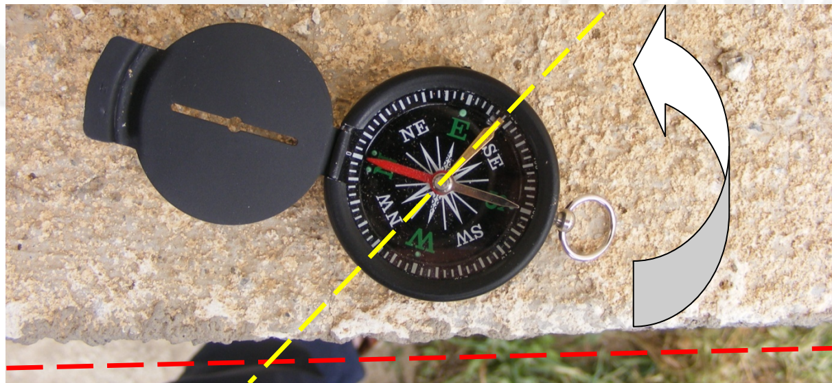
Fig. 13.4 Compass placed in the foundation of the mosque, note the golden arrow with (or yellow line) that shows the direction that Mosque should be directed, respectively, in this case the foundation ring (red line)
