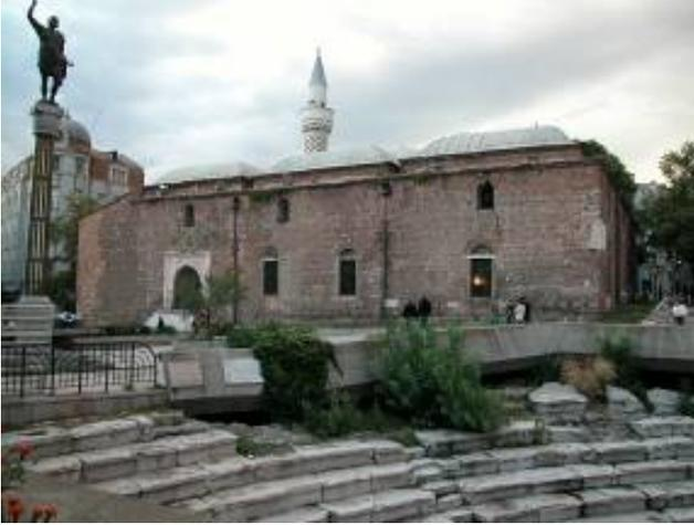
**This angle shows part of the excavated Roman amphitheater. Excavation exacerbated a subsidence problem that threatens the structural integrity of the mosque. The execution of the excavation during the 1970s may have been as much as a political statement to diminish the stature of a “Turkish” monument as it was scientific in its motivation.**
