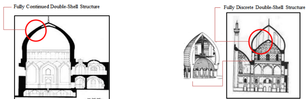
Figure 64: Fully continued and discrete double-shell dome structure. (Amoli, Mohammad Reza, 2011)
