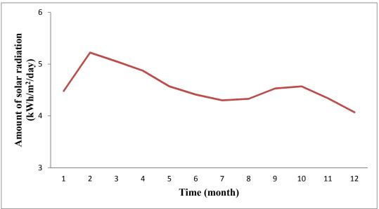
Figure 1. Monthly radiation incident average on a horizontal surface for 2008 (kWh/m²/day) [6]
