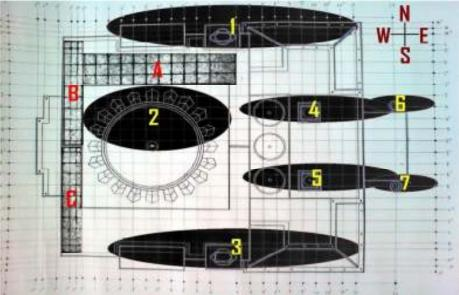
Figure 3. Shading and suitable area for PV installation
