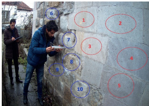
Fig. 4 Surface hardness measurement
