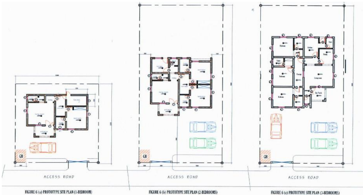
Figure 6 (a-c). Showing an architectural design proposal of a one-bedroom apartment (a) to address requirements for the lowest income group on the plot size of 225m 2 , and to maintain uniformity of design with the two and three bedrooms, (b & c) the proposed house has same footprint area of living room, first bedroom, and its toilet, guest toilet, corridor and lobby. (Source: Design by Author, 2018)
