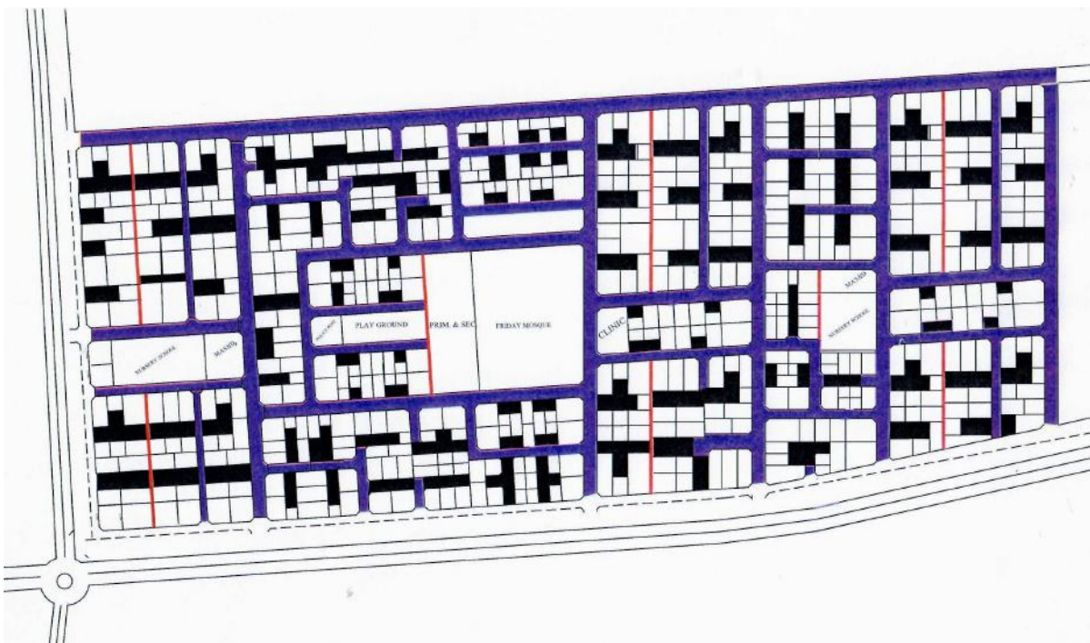
Figure 4. The redesigned Site layout from Gridiron to Cluster housing pattern to achieve the concept of ‘ Ummah .’ The concept of Ummah aims to promote social cohesion, brotherliness, communality and participation among residents, an essential requirement on Islamic housing neighborhoods. (Source; Redesign by Author, 2018)
