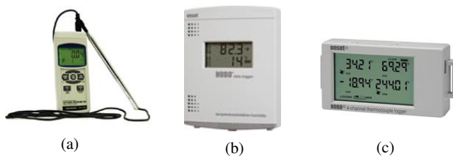
Figure 3 (a) Hot Wire Anemometer with Data Logger; (b) HOBO Temperature/Relative Humidity Data Logger; and (c) HOBO UX120 Series Data Loggers.
