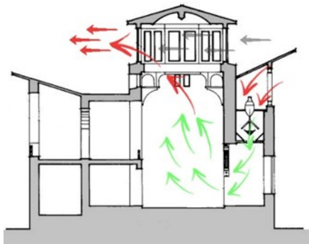
Figure 1: The example structure for a passive cooling tower system by Hassan Fat'hi
