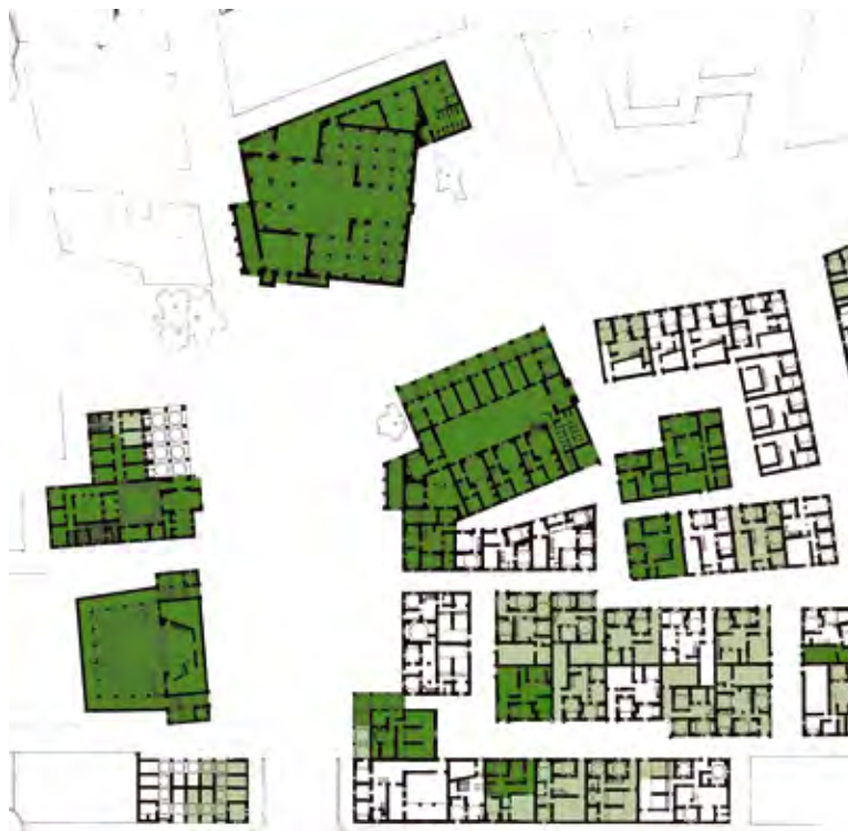
The buildings of New Gourna recorded to be original by UNESCO in 2010 (dark and light) and the ones that still had significant original or reconstructed/rebuilt parts in 2019 (dark)
