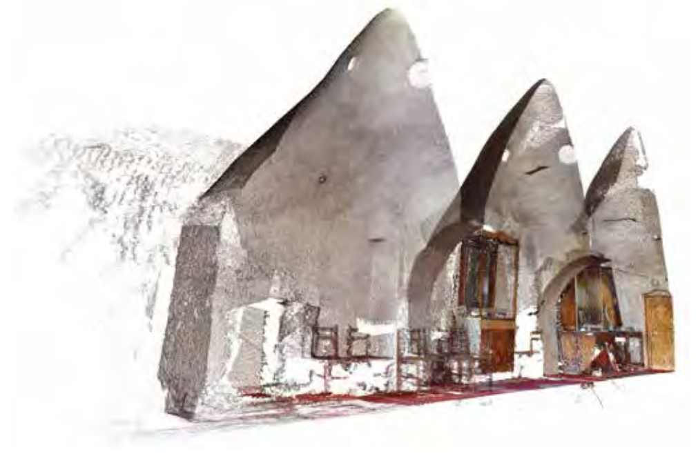
Section of a series of domes of the St. Tawadros Monastery (3D pointcloud, SfM). Compiled by B. Miklós based on data captured in 2017-2018.
