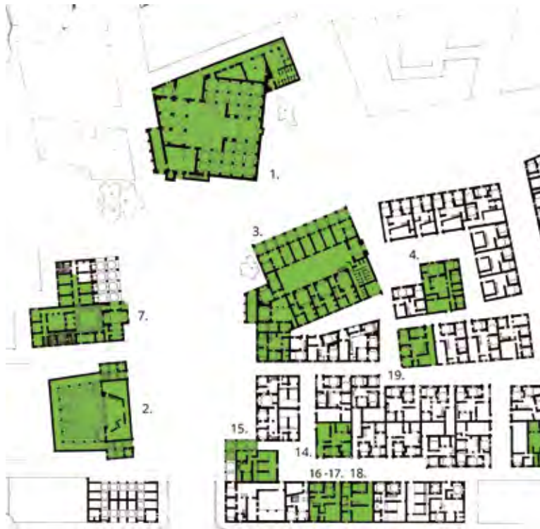
The buildings of New Gourna documented by the Hassan Fathy Survey Mission between 2015-2019, which still had significant original or reconstructed/rebuilt parts of the original structures.
