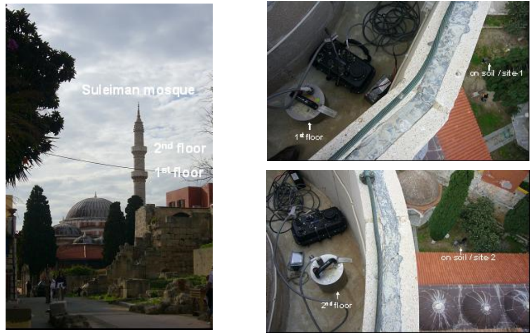
Figure 6. The instruments were placed on the ground soil and on the two balconies of the minaret [52].
