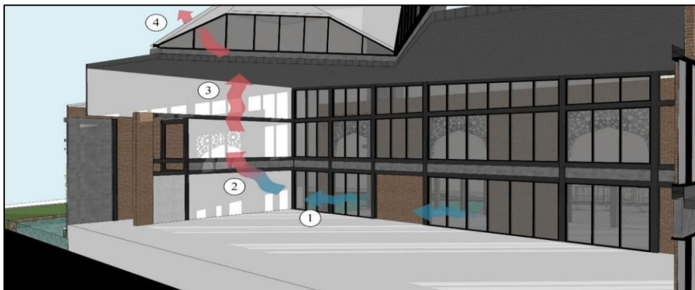
Figure 14. Three-dimensional (3D) cross section model with natural ventilation diagram.
