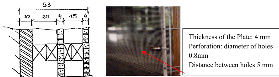
Figure 13. The two layer glass along with its specifications.
