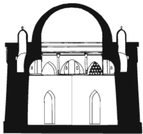
Figure 253: Isma'il Samanid mausoleum Section
